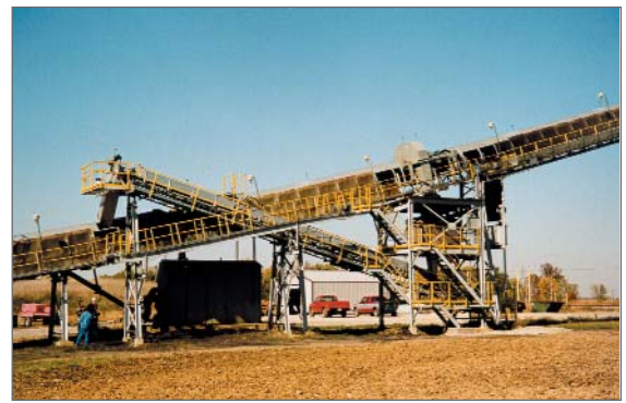
A sampler feeds coal to the COALSCAN 9500 and a conveyor returns the coal to the main belt.
